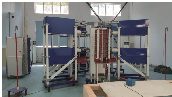
Fig 5. Lightning surge tests for LMS-W in Shanghai lightning protection center.
